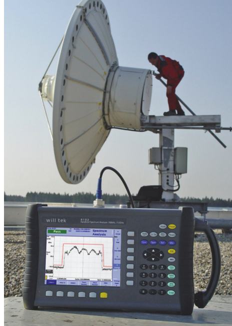
When selecting a spectrum analyzer for field use, a bright screen is an advantage. The Model 9201 from Willtek includes a high-contrast display readable in direct sunshine. Courtesy of Willtek.
