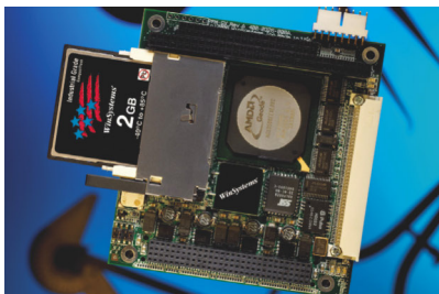
The PPM-GX, a PC/104-Plus compatible single-board computer, sports an Ethernet controller, four UARTs, and two USB ports. Courtesy of WinSystems.
