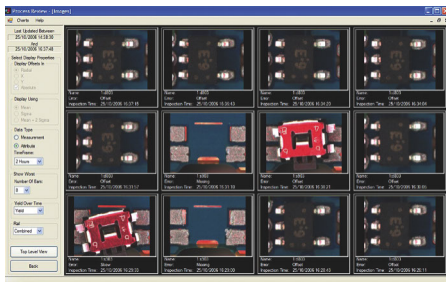
These images reflect worst-case results from a series of production runs. Courtesy of Agilent Technologies.
